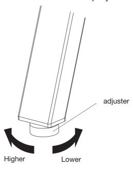
To keep the desk and the floor level, adjust it with the adjuster.
