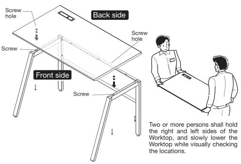
Place the Worktop while inserting the screw heads to the screw holes (one each on right and left sides).
