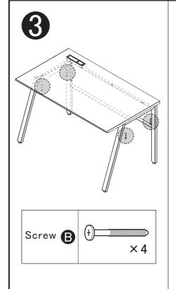
Tighten Screw **B** from the upper bottom side of the Leg to fix the Worktop to the leg (four locations).
