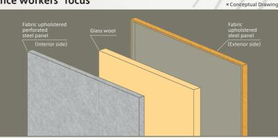
The slim profile panels are only 1 3/16" thick. The core of these panels have glass wool insulation for excellent sound absorption. The clean and straightforward design creates mini-environments for focus throughout the office while also adding aesthetic interest points and color to the workplace.
